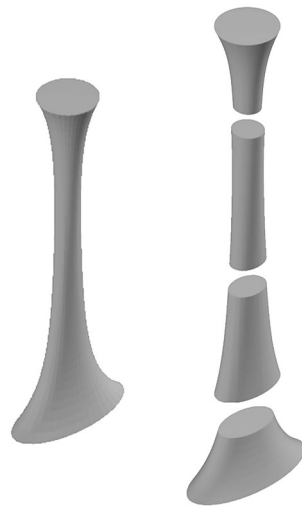
Figure 1. 3D model of case-study pillar (left); the pillar broken down into four pieces that can be printed with the HINDCON demonstration plant.
