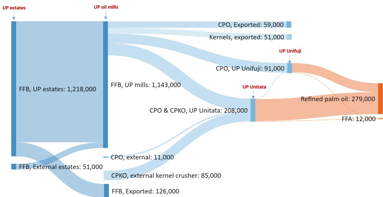
**Figure 1.2:** Sankey diagram of the flows of United Plantations in 2020, through their estates, oil mills and refineries. The product portfolio includes "CPO exported", "Kernels exported", "Refined palm oil" and "FFA". The FFA (free fatty acid) is also sometimes referred to as palm acid oil (PAO).
